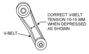
Figure 8. V-Belt Tension
